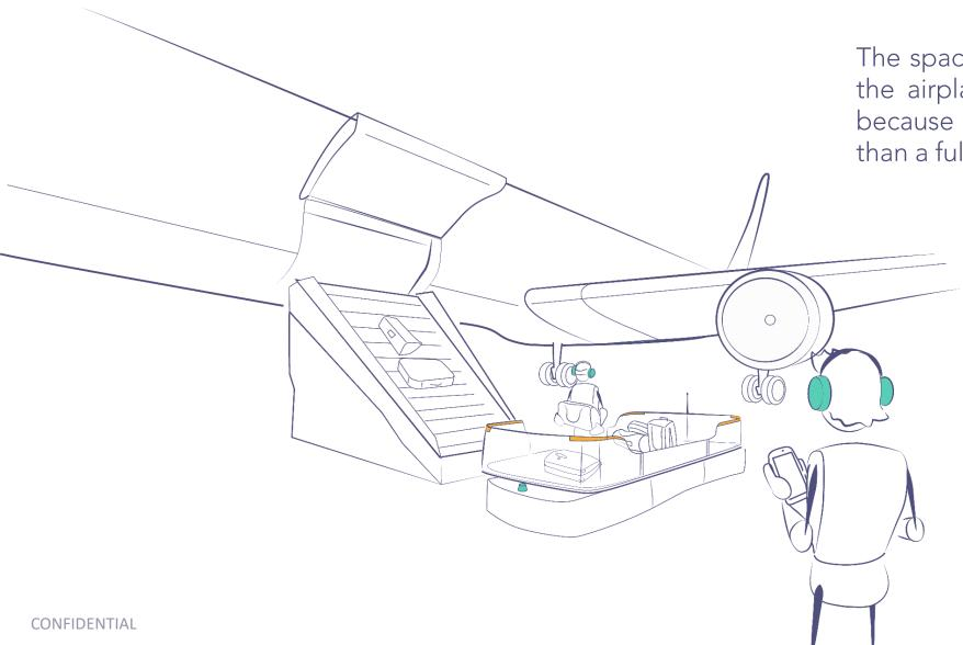
The space occupied by the robots near the airplane baggage hold is reduced because a robot takes up less space than a full train.
