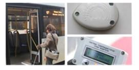
passenger's desire to board. A source of sound signal is installed above the vehicle door to help the disabled person determine the exact location of the door.
