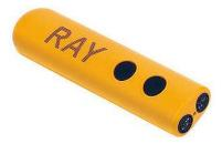
The ultrasound cane is a small, portable and lightweight device (50 g) powered by 2 rechargeable batteries and fits in any pocket. The obstacles can be recognized at distance of up to 2.85 meters, and the device will notify its owner about this by means of a sound signal or vibration (the user can choose between these two modes).
